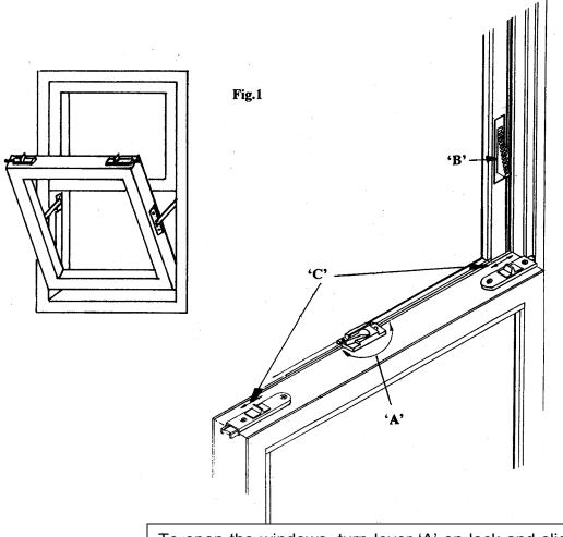
To open the windows, turn lever 'A' on lock and slide the bottom sash up or the top sash down.
